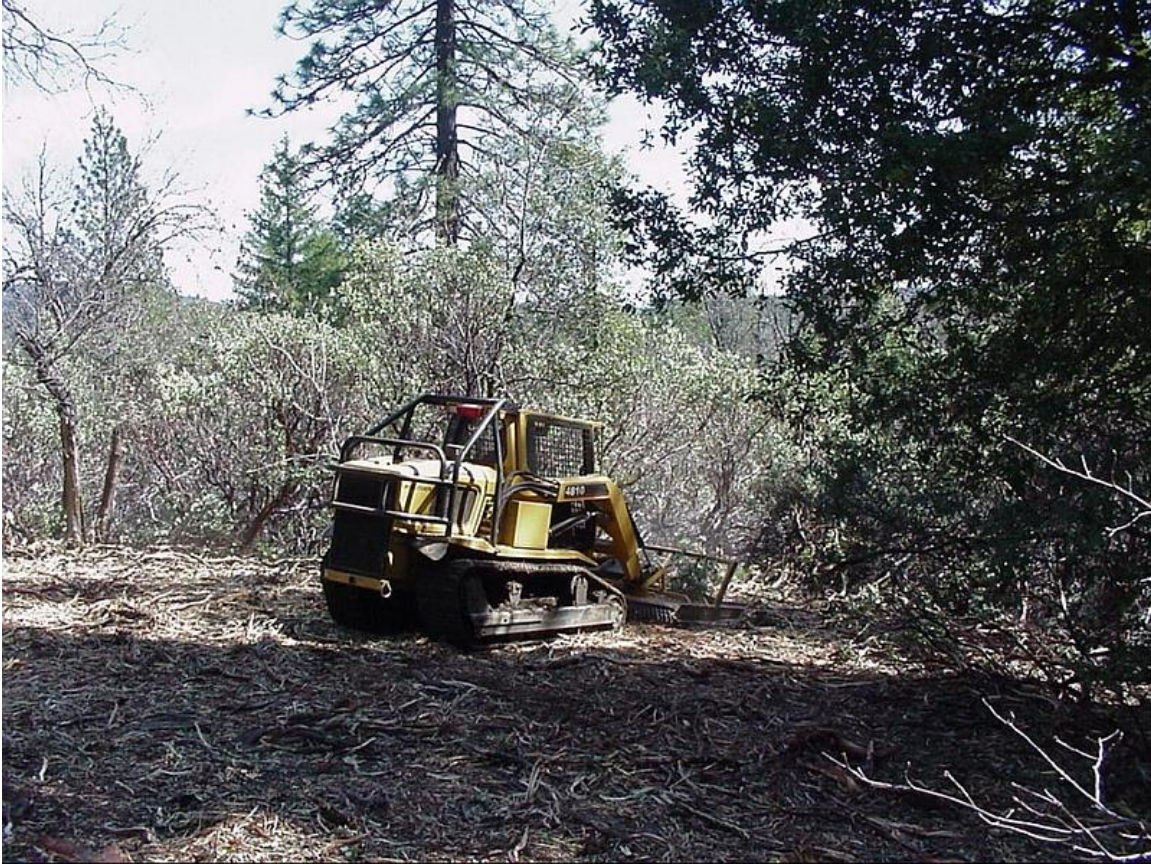
Mastication using a track loader and mower head
